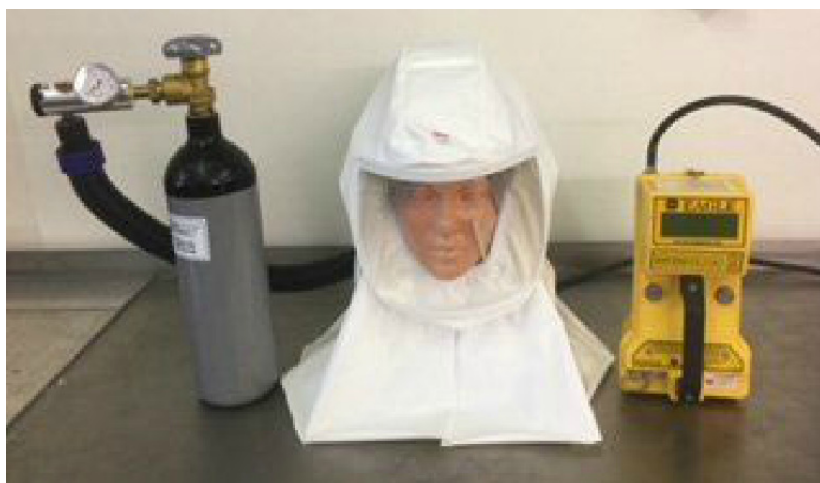
Nitrogen delivery to the 3M Versaflo S-533L helmet & gas analysis
