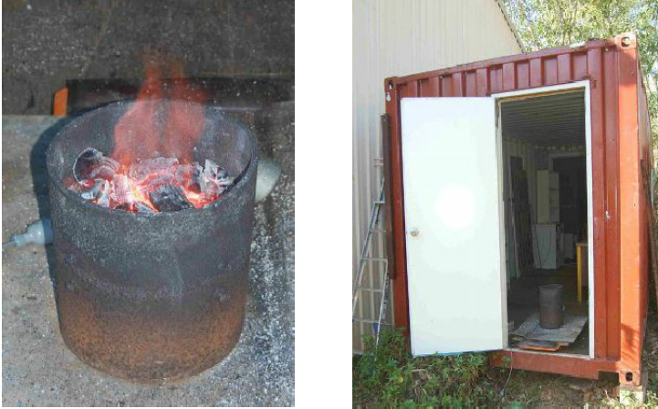
Fig 6.10. Charcoal burner, brazier and test shipping container
