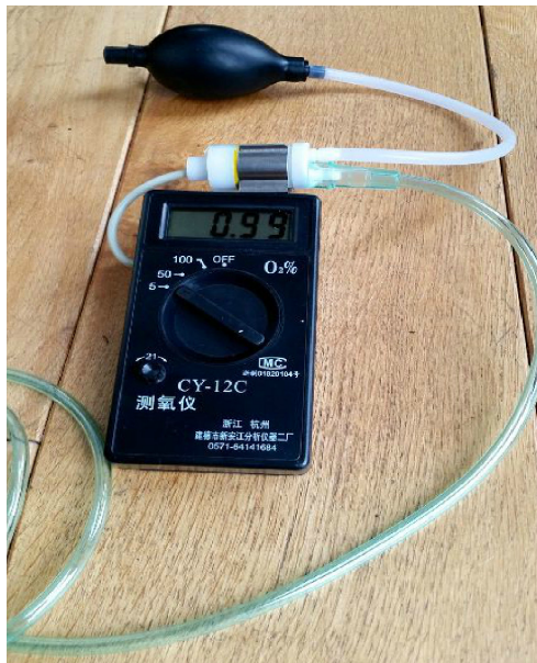
Oxygen Meter used to detect gas contamination see 'Gas Purity Testing'
