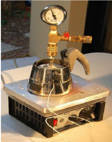
Fig 20.2 (above): The 'Single Shot' Autoclave A: Pressure Gauge B: Distillation coupling C: Pressure coupling D: Pressure safety valve E: Heat + Stirring F: Thermocouple G: IR thermometer patch
