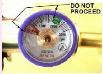
Fig: Checking gas pressure
