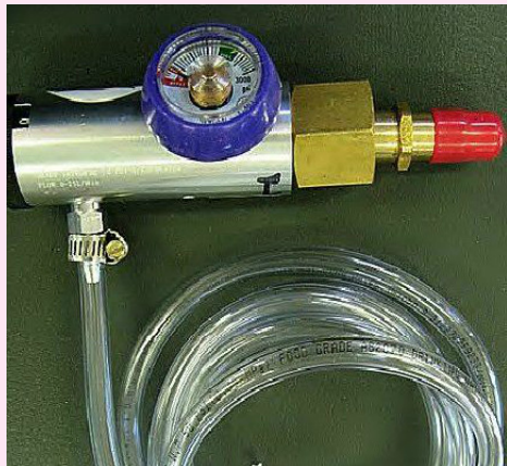
Fig: 6mm PVC tubing attached to a MaxDog gas regulator
